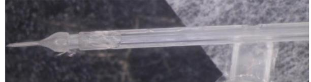
Fig 2 Result of insert molding
